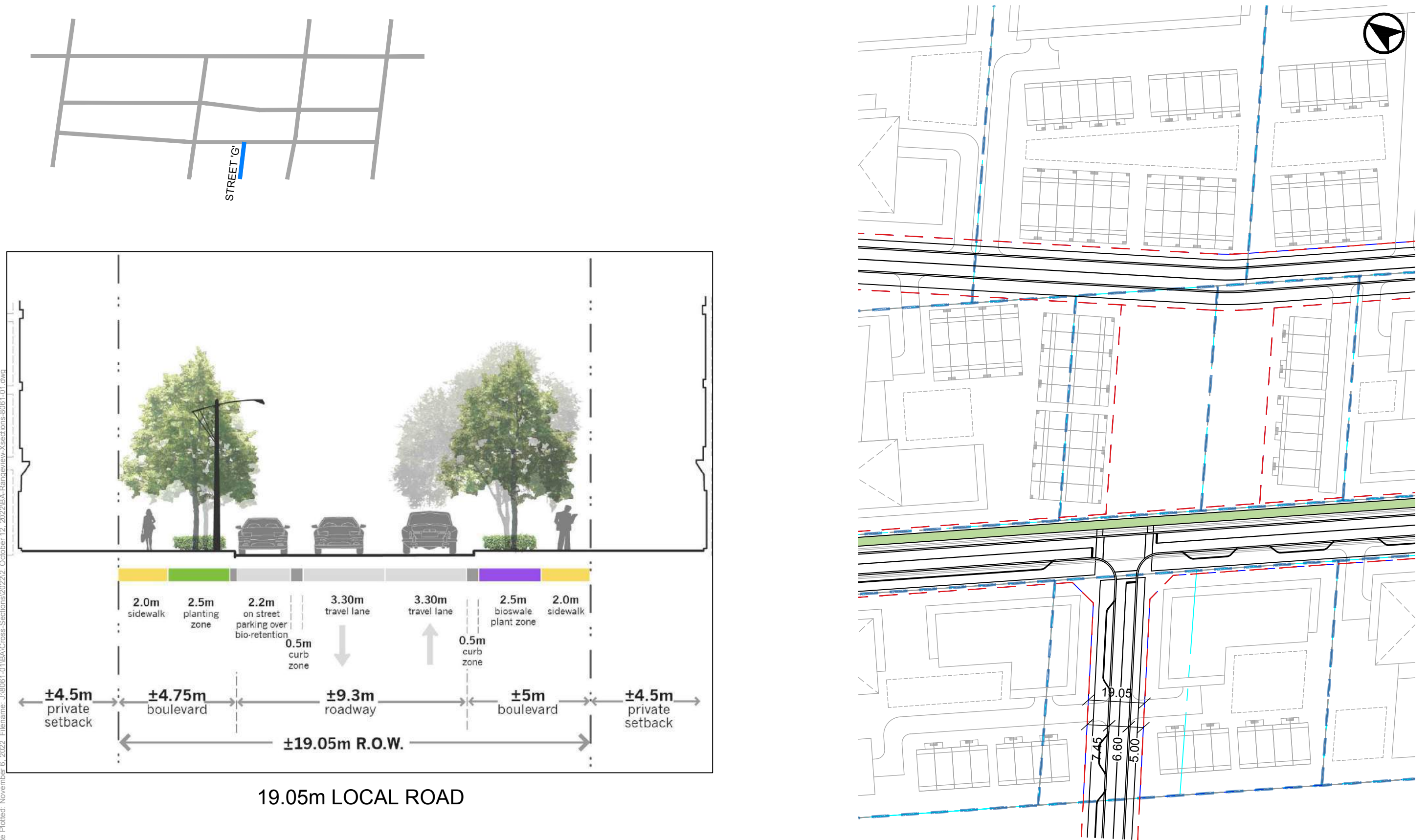
FIGURE 12 PROPOSED STREET 'G' EXTENSION - FUNCTIONAL PLAN & CROSS-SECTIONS
