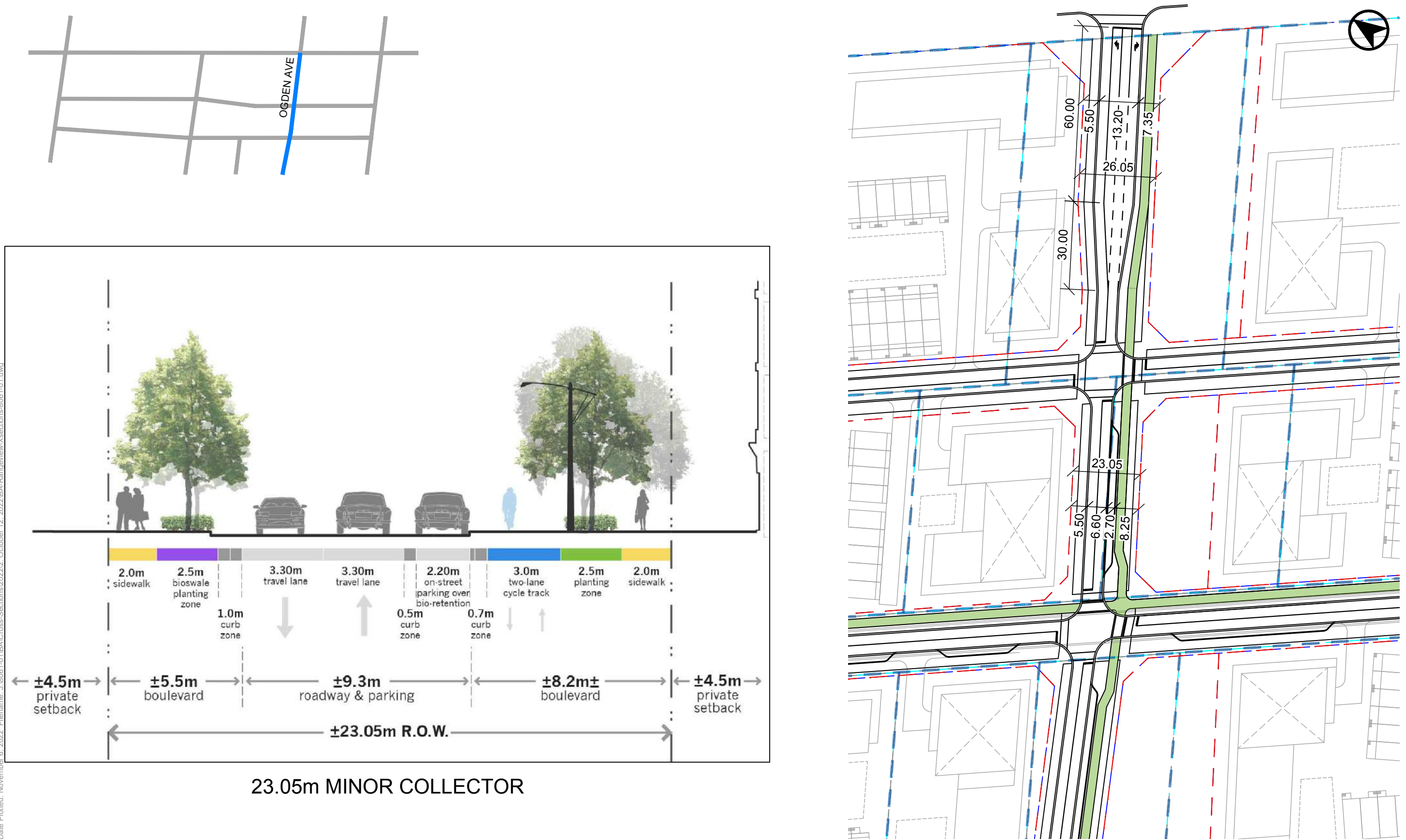
FIGURE 8 PROPOSED OGDEN AVENUE EXTENSION - FUNCTIONAL PLAN & CROSS-SECTIONS
