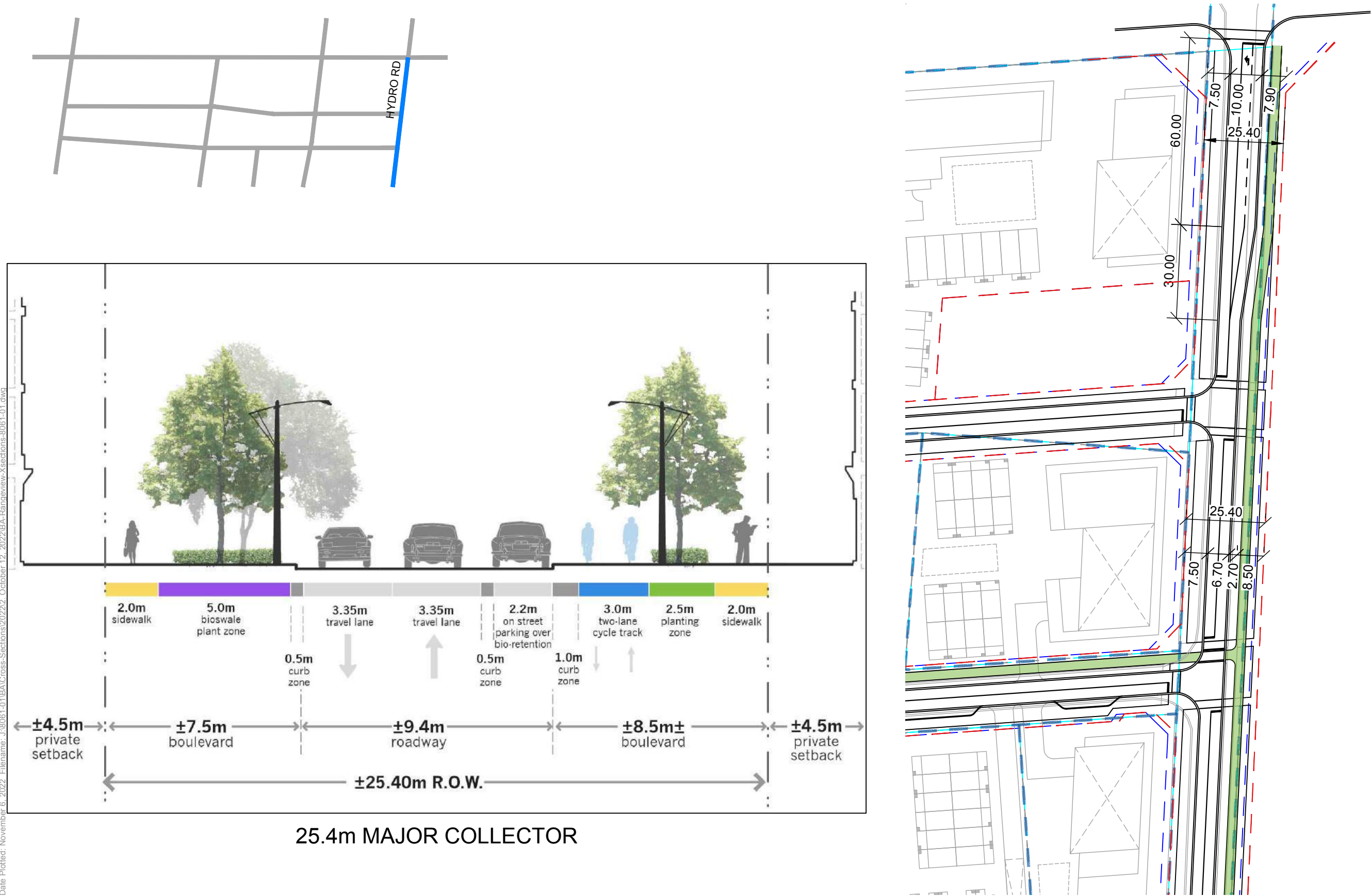
FIGURE 9 HYDRO ROAD - FUNCTIONAL PLAN & CROSS-SECTIONS
